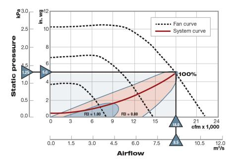
Figure 3: FEI Bubble Curve for 18-in. (464-mm) Backward-Inclined Fan Showing Compliance at Low Flow Rates, but not at the Peak Design Condition
