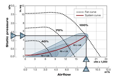
Figure 4: FEI Bubble Curve for 22-in. (565-mm) Backward-Inclined Fan Showing Compliance at all Three Duty Points of Interest
